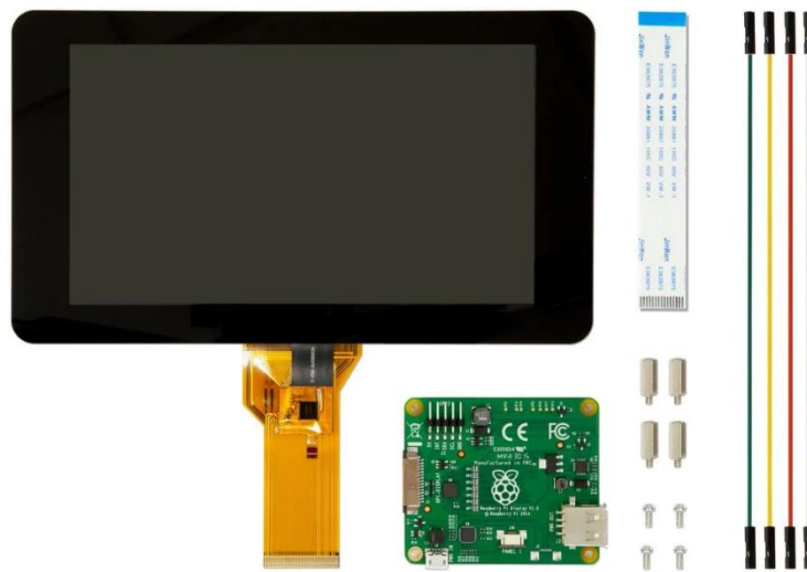
Figure 2.7 Raspberry pi Touch Screen [25]
